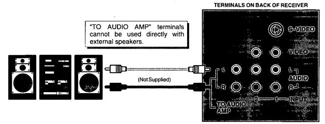
Adjustment - When an audio amp is connected to "TO AUDIO AMP" terminals:
